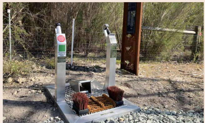
Boot cleaning station for dieback hygiene.
